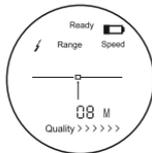
**Note:** If the battery indicator icon shows up, the battery should be replaced immediately – failure to do this may mean that measurements are not accurate. Remove the battery if the unit will not be used for a long time.
